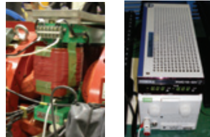
Fig. 2. Photographs of additional equipments. Left: Additional small coil around the steering magnet. Right: Remotely controllable DC power supply.
